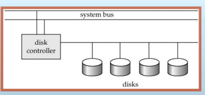
Multiple disks connected to a computer system through a controller
