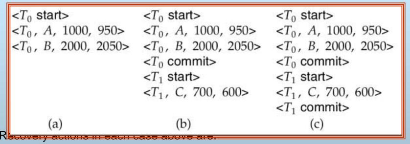
(a) undo  $(T_0)$ : B is restored to 2000 and A to 1000.
